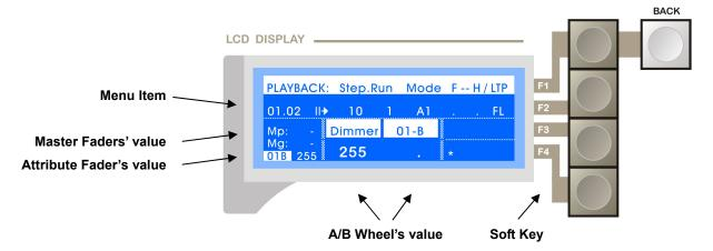
The menu is operated by Soft Keys, which is easy and fast.
